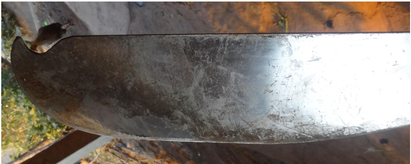
FIGURE 9: THE IMPROVED KOITA. NOTICE THE BARB AT THE TIP OF THE BLADE
