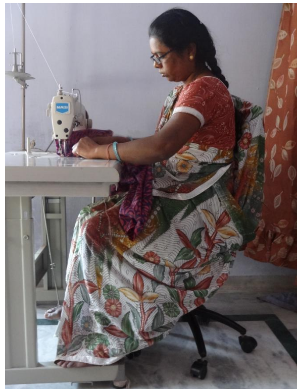
FIGURE 2: CHAIR USER WHO MODIFIED THE SEWA CHAIR BY ATTACHING WHEELS ON THE STAND
