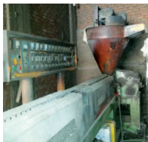
Figure 46. Large trader's equipment to melt plastic.
